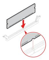
**Note:** During the installation, ensure that you align the memory module to the slot and press down on both ends until the latches are fully engaged with a click.
