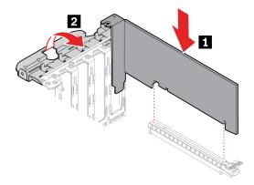
**Note:** During the installation, ensure that you align the PCI-Express card to the slot and press down until the latch is fully engaged with a click.
