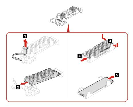
**Note:** When installing the M.2 solid-state drive and the heat sink, remove the film (if any) that covers the thermal pad.
