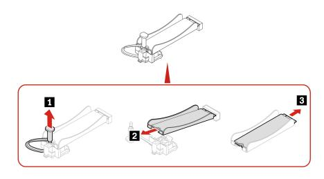
**Note:** When installing the M.2 solid-state drive and the heat sink, remove the film (if any) that covers the thermal pad.
