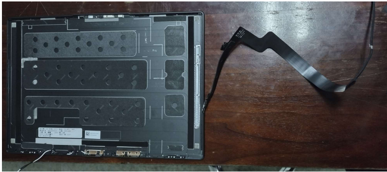
Figure 24. Remove the camera cable
