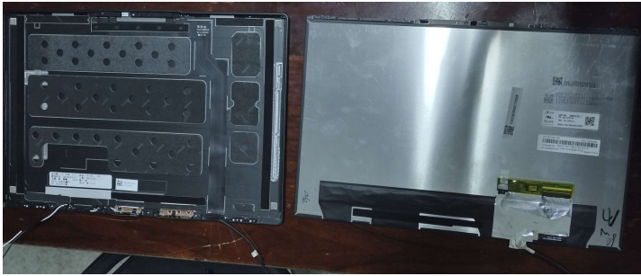
Figure 21. Remove the LCD panel
