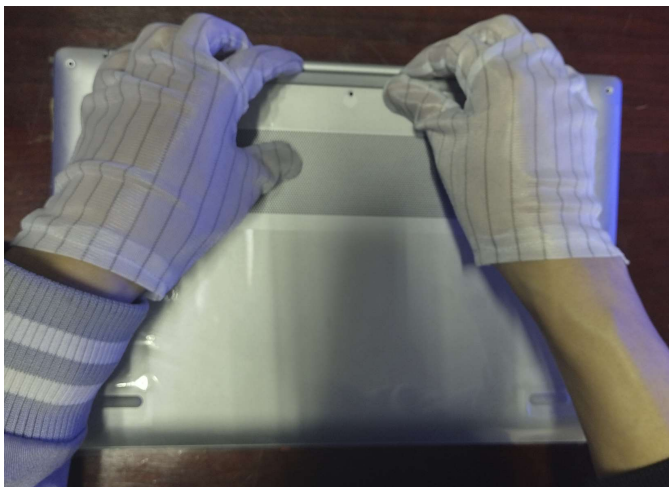
Figure 4. Pry up the latches and remove the lower case
