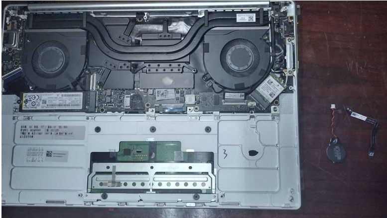
Figure 8. Remove the CMOS battery
