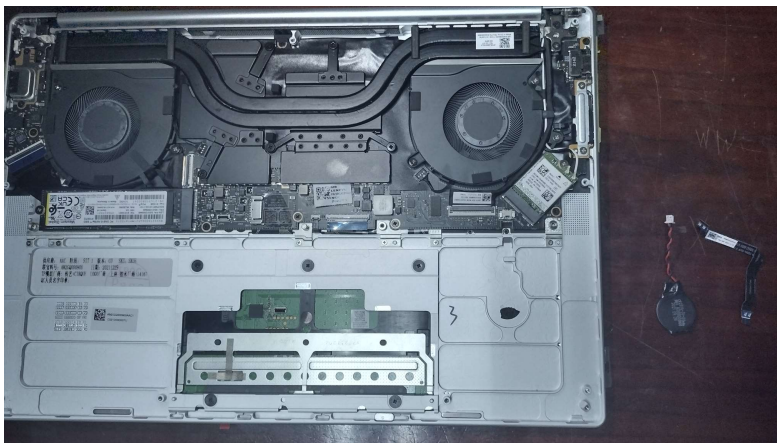
Figure 7. Remove the touchpad cable
