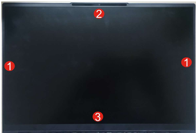
Figure 20. Remove the LCD bezel
