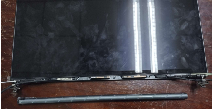
Figure 17. Remove the hinge cover
