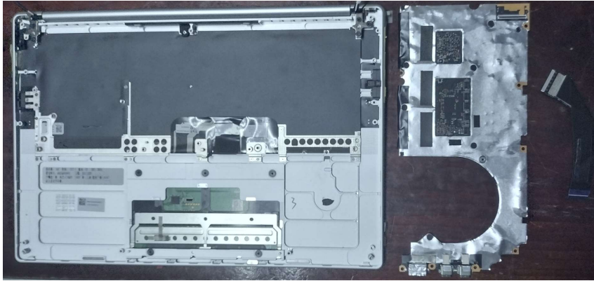
Figure 15. Remove the I/O board cable
