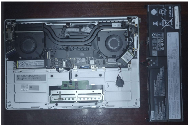
Figure 5. Remove the battery pack
