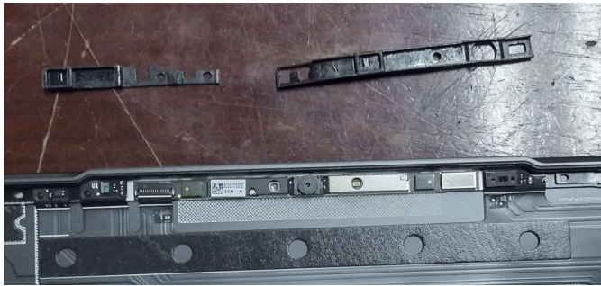
Figure 23. Remove the camera rubber
