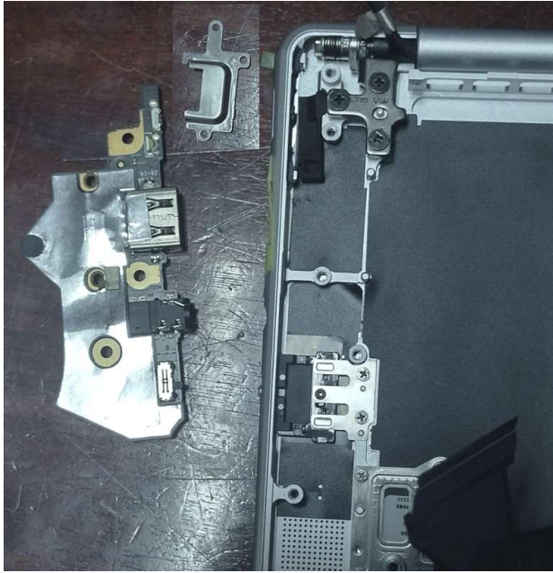
Figure 14. Remove the I/O board
