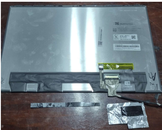
Figure 22. Remove the EDP cable
