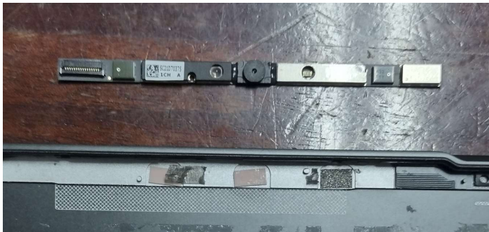
Figure 25. Remove the camera board
