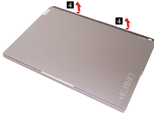
Figure 31. Remove the strip cover
