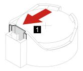
4. Remove the coin-cell battery.
