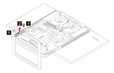
4. Remove two screws and then remove the power switch bracket.
