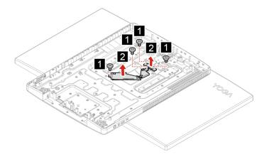
4. Remove four screws. Then, remove the base support assembly.
