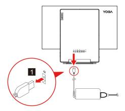
3. Remove the power cord from the ac power adapter.
