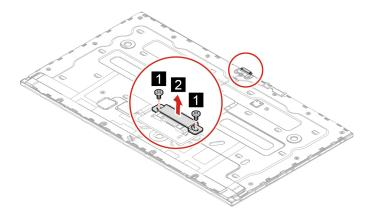
3. Remove two screws that secure the microphone board bracket.
