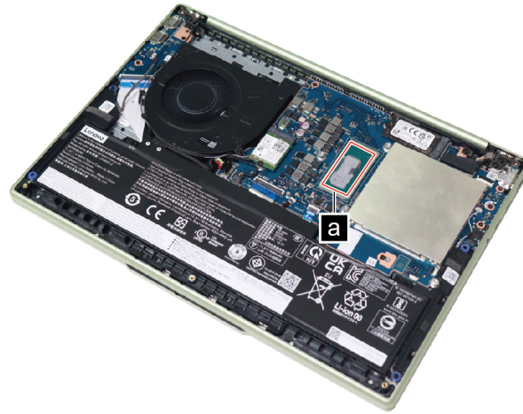
Figure 5. Areas on the system board where thermal interface materials are applied (for Intel models)
