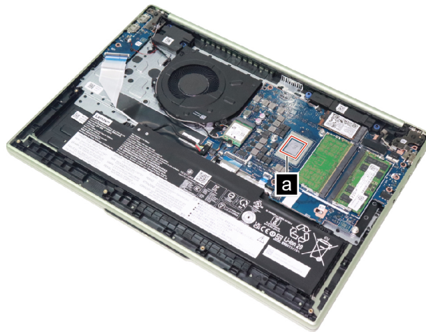
Figure 6. Areas on the system board where thermal interface materials are applied (for AMD models)
