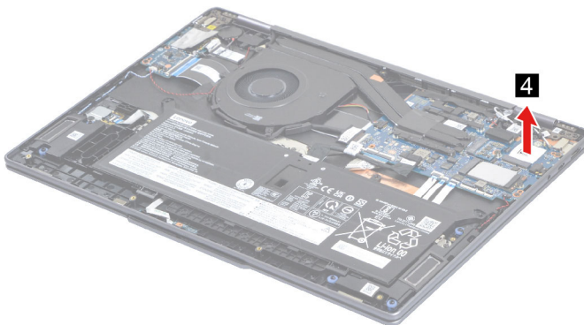
Figure 18. Remove the Wi-Fi card thermal pad
