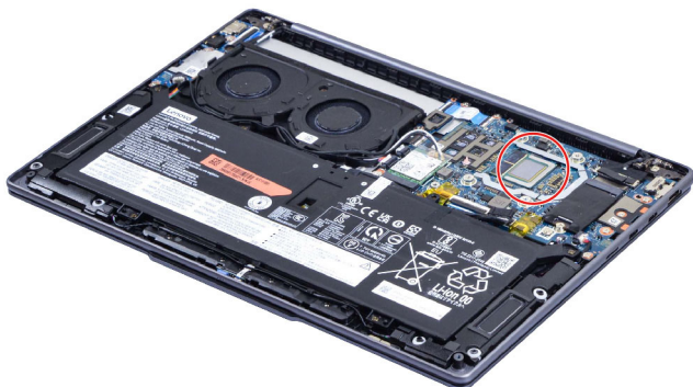
Figure 4. Areas on the system board where thermal interface materials are applied—Yoga Slim 7 14ILL10
