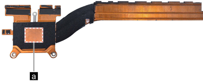
Figure 3. Areas on the heat sink where thermal interface materials should be applied—Yoga Slim 7 14AKP10
