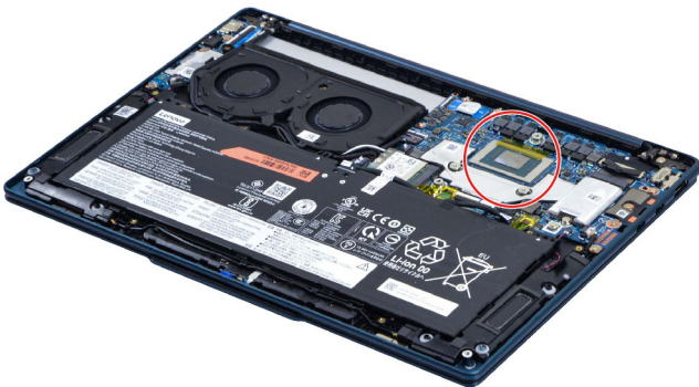
Figure 5. Areas on the system board where thermal interface materials are applied—Yoga Slim 7 14AKP10
