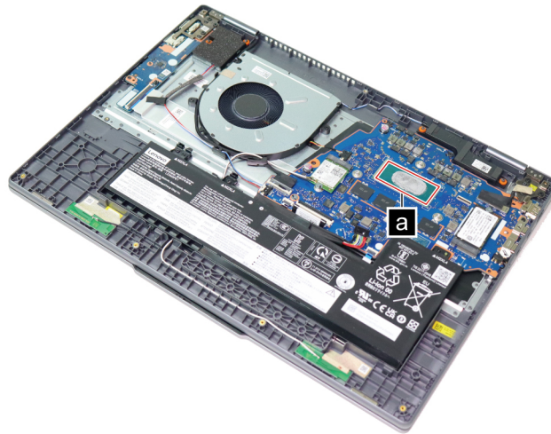
Figure 5. Areas on the system board where thermal interface materials is applied (for Intel models)
