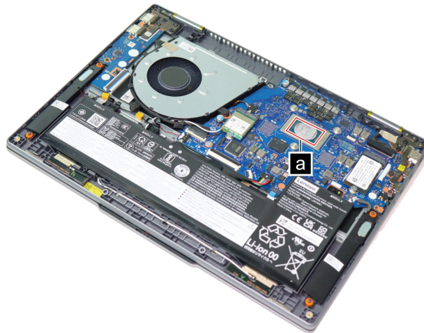
Figure 4. Areas on the system board where thermal interface materials is applied (for AMD models)
